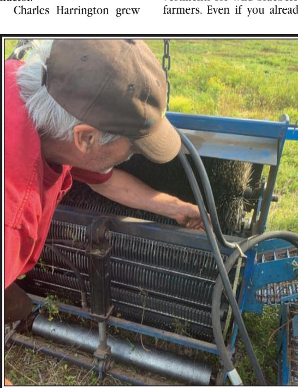
Hand rakes have been replaced by harvesters in the wild blueberry fields but the concept of metal teeth gently pulling the berries from the vines is similar. Charles checks over the "teeth" to make sure none are bent or broken.
