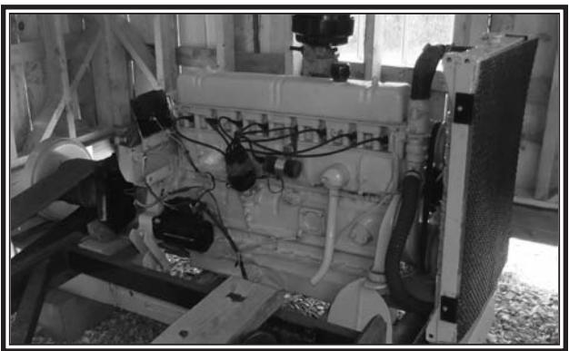
A new engine has been purchased and installed to power the sawmill. (Rees Photo)
