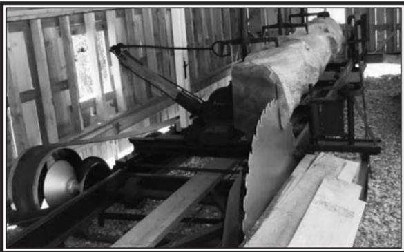
The blade started to make a cut, but the blade needs to be raised to penetrate the full diameter of the log. (Rees Photo)
