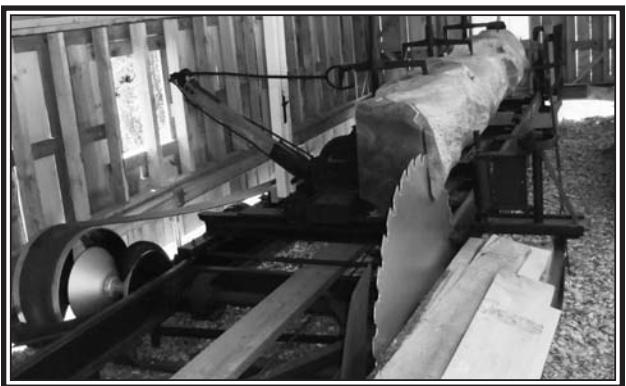
The blade started to make a cut, but the blade needs to be raised to penetrate the full diameter of the log. (Rees Photo)
