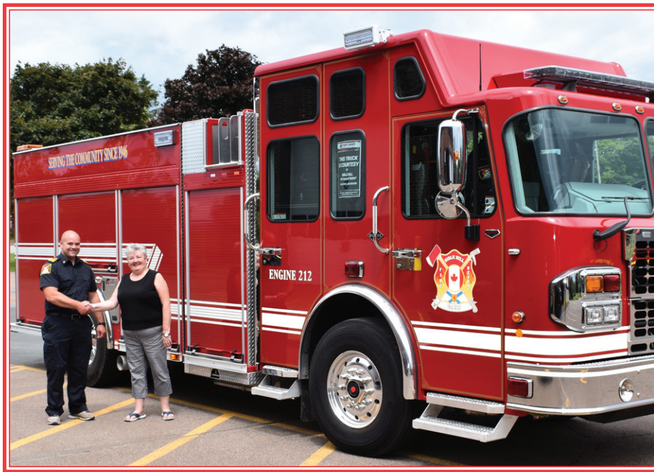
Village of Bible Hill's has accepted delivery of its new custom built 2019 Spartan Metro Star Pumper Tanker built by Fort Garry Fire Trucks of Winnipeg. Features of the truck include: 20" raised roof, 400 horsepower Cummins diesel engine; Allison automatic transmission; 4,542 litre poly tank and a side mounted pump that delivers 4,731 litres per minute at 150 PSI. On hand for the acceptance ceremony were Fire Chief Joey Bisson and Bible Hill Village Commission Chair, Lois MacCormick. (Submitted)
