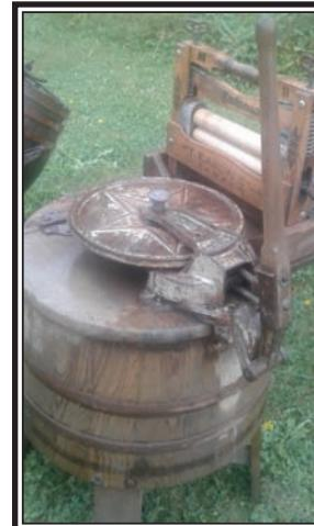
Pull the handle to turn the agitator to wash the clothes, slide the cover aside then turn another handle to put the clean clothes through the wringer. Didn't need electricity and the laundry person was the source of power. (Rees Photo)
