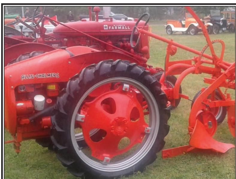
The engine on the rear provided increased traction for this Allis Chalmers dedicated motorized plow to give the driver a ride instead of following a team of horses. (Rees Photo)
