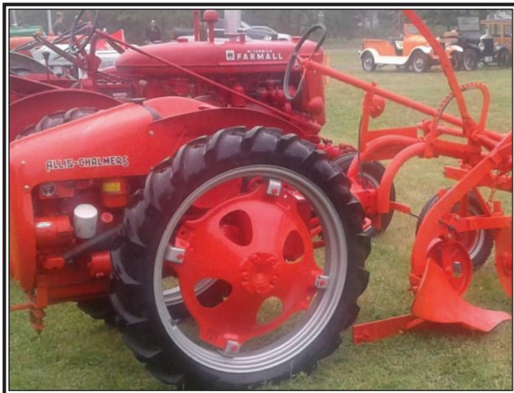
The engine on the rear provided increased traction for this Allis Chalmers dedicated motorized plow to give the driver a ride instead of following a team of horses. (Rees Photo)
