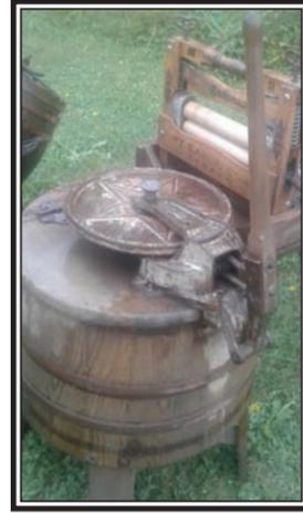
Pull the handle to turn the agitator to wash the clothes, slide the cover aside then turn another handle to put the clean clothes through the wringer. Didn't need electricity and the laundry person was the source of power. (Rees Photo)
