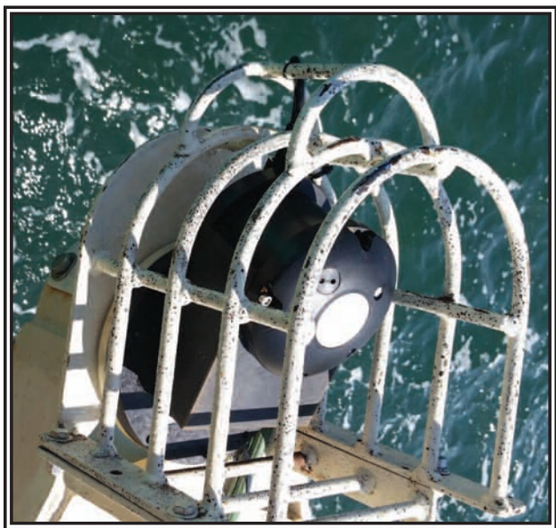
Acoustic sensors on the FAST-1 monitoring platform are protected by special cages on all corners of FAST1 platform. (Image: FORCE)
