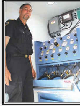
Debert Fire Chief Wade Jennings checks out the eight bottle cascade air system on the new truck. It is capable of filling three oxygen bottles at a time.
