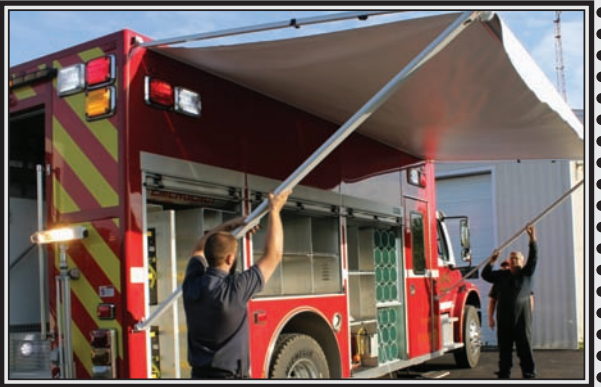
Debert Fire Brigade's new truck has an awning attached to the side which can provide shelter during emergency calls.
