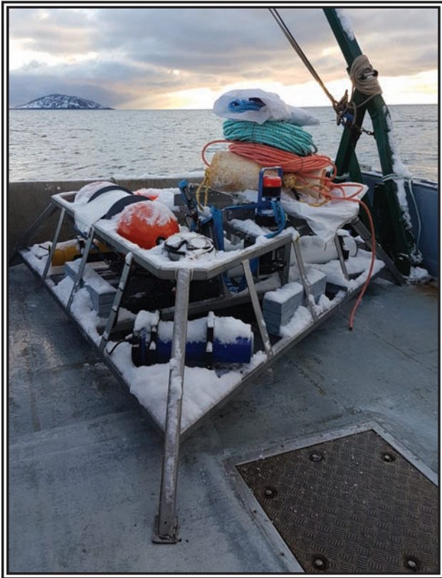
FAST-3 underwater sensor platform gets ready for deployment near the FORCE test site in the Minas Passage, NS.
