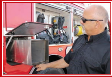
Carl Gallant opens the compartment for one of the two water side dump ports.
