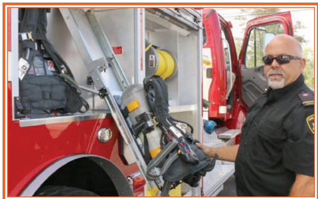
Lantz Truck Body designed a slide out for the back pack self-contained breathing apparatus. One of the many features on the 'Half-Million Dollar Fire Truck' recently delivered to a very appreciative Onslow-Belmont Fire Brigade. See the story and more photos on pages 16 and 17 of this Shoreline Journal.
