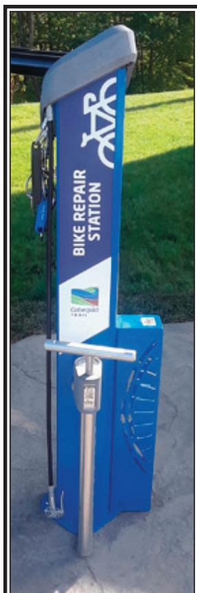
With an emphasis on cycling bicycles always are in need of repair. This bicycle repair station is state-of-the-art complete with pump, repair rack and a few wrenches. (Rees Photo)
