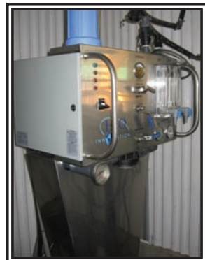
Reverse osmosis is used to extract most of the water from the sap. Currently Matthew Harrison is investigating using the purified water either in a bottling operation or sold in bulk to craft brewers. (Rees Photo)
