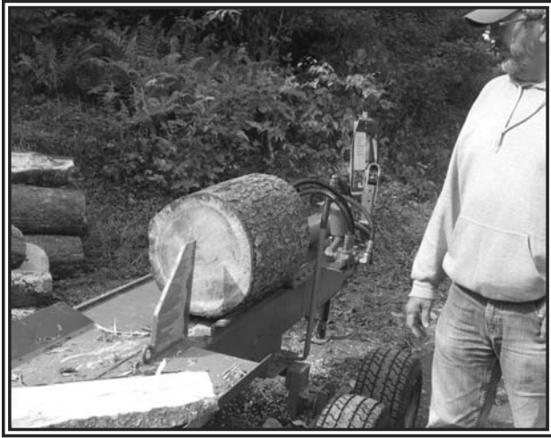
Walter Rodler has modified this wood splitter so that a rail holds the stick of wood in place, installed a new knife instead of the original wedge and by reversing the pump a quick push of a lever activates the splitting process. No hands are required to hold the wood in place, eliminating the possibility of losing a finger or hand in the process. (Rees Photo)
