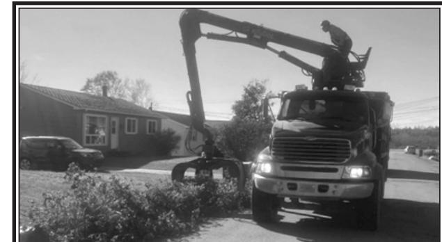
Phil Redden, who Colchester contracted to head up the Fiona Clean-up team chose several grapple loader trucks to handle larger debris and to expedite the clean-up process with grapple trucks rather than removing debris by hand into compactor trucks. Loader operator can be seen checking to ensure he is not damaging curbs or edges of the lawn. (Redden Photo)
