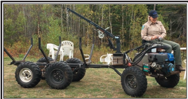
Amelia Kennedy takes a turn at driving Norm's Buggy, which he designed and built to carry approximately 1/2 cord of random length wood. (Submitted)
