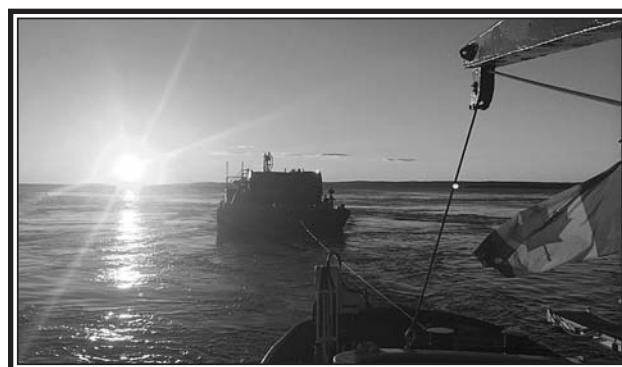
It was a long workday on Sunday, October 21st, with the sun setting on the barge laying the underwater cable in Minas Passage. The area contains the highest and most turbulent tides in the world. The turbines will immediately start generating electricity when they are connected to the cable in 2015. (Submitted)
