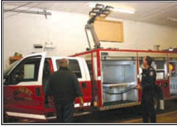
Lots of new gadgets to try out! Fire Chief Wade Jennings raises the telescopic command light on top of the new truck, while Shane Slack looks on. (Harrington Photo)
