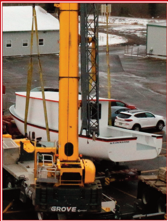
Within minutes of arrival, heavy duty straps were secured under the 5 1/4 tonne boat, Ready for liftoff.
