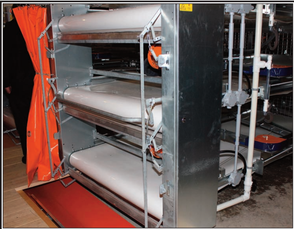
The automated manure removal system, easily cleans waste from beneath cages and uses a 24" inch conveyor belt, supplied by Northumberland Silos, to move the material out of the building.
