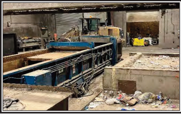
As shown above, staff removed the hopper and stripped the baler apart down to the bones and a crew from the Marathon Dealer in Moncton arrived on site January 28th to start going over all of the welds, repairing what is damaged, as well as fixing anything that looks like it may cause a problem in the future. While it is apart they will also be replacing the chamber wear plates and performing any other needed maintenance during the shutdown. (Colchester Photo)
