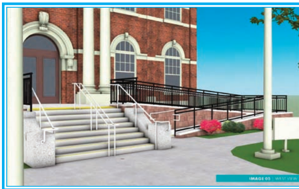
These graphics illustrate preliminary schematics of the proposed work to install an accessibility ramp at the front of the municipal building at 1 Church Street. (Colchester)
