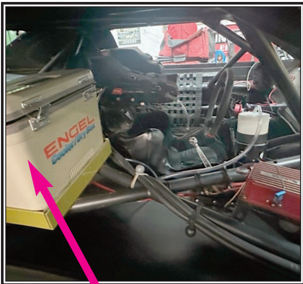
In the heat of summer, temperatures inside the race car soar. To prevent heat exhaustion, cars are equipped with a cool box which circulates cold water through the driver's cool suit to keep body temperatures down.
