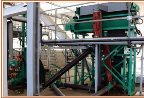
A roller press produces greener bedding, reducing waste material.
