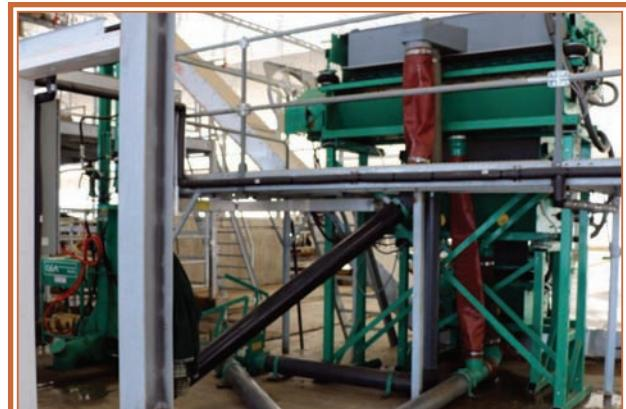
A roller press produces greener bedding, reducing waste material.
