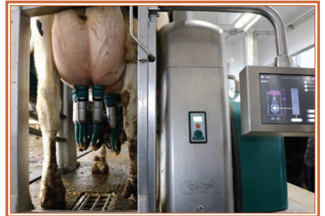
When a cow steps into the milking parlor, a 3D camera is used to automatically hook a cup to each of the four teats.
