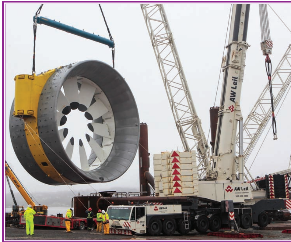
A 650 tonne crane is used to place the center of the turbine into the outer shell at the Pictou Shipyard, Pictou. The outside diameter is 16 meters (52.5 feet), while the inside holding the blades is 14 meters (45.9 feet). (Darren Pittman/Images East Photo)
