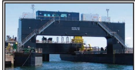
The Scotia Tide a catamaran-style barge with a capacity of 650 tonnes sits at the wharf awaiting its call to transport the turbine around Cape Breton, then around Yarmouth up to the FORCE site near Parrsboro during a 2 week trip. The Barge was built in Pictou and its sole purpose is to transport Open Hydro's two turbines. (Rees Photo)
