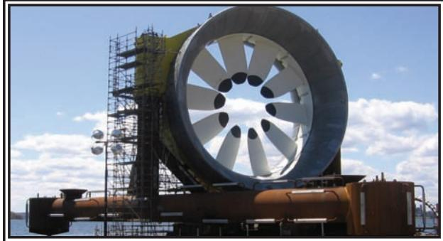
Almost ready to be loaded onto the Scotia Tide Barge, the turbine rests on the end of the marine railway at Pictou Shipyard. Photo taken on May 19th during a media tour granted by Cape Sharp Tidal. The outside diameter is 16 meters, while the inside holding the blades is 14 meters. (Rees Photo)
