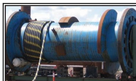
This large braking drum winch holds a portion of the undersea cable which will extend from the turbine to the "hub connection", which was installed last year, when FORCE installed the undersea cable to connections on land (Rees Photo)
