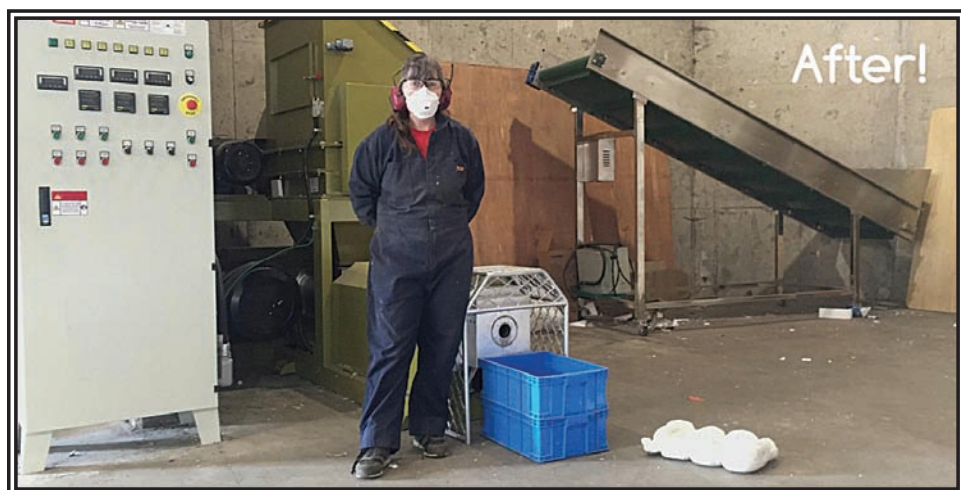
The small pile on the floor beside Dawn Rafuse is what was left after she performed her duties of putting the Styrofoam through the thermal densifier. Residents and business owners can see how much they will help save space and reduce landfill costs, if they recycle all the Styrofoam in their possession. (Submitted)
