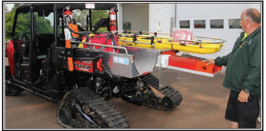
OBFB Chief Greg Muise checks out the stokes basket and pull out storage shelf added to the Medlite transport unit on the back of the Polaris 900 Ranger Crew. The new vehicle is a 4 season multi-purpose unit giving the Brigade greater access to remote or compromised locations. (Harrington Photo)
