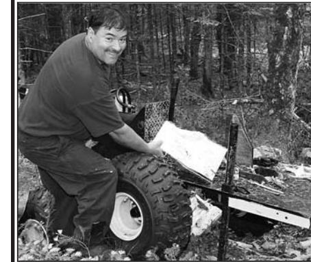
This all-terrain wood splitter can go anywhere the going gets rough. Walter Rodler demonstrates how even on this hilly terrain the splitter stays level, making a perfect cut even through knotty wood.
