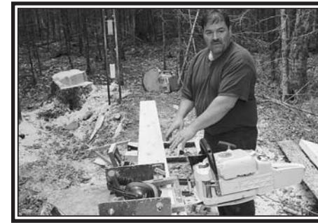
Walter Rodler shows how one of his inventions can turn an ordinary powersaw into a portable saw mill to create finished lumber right where the tree has fallen.
