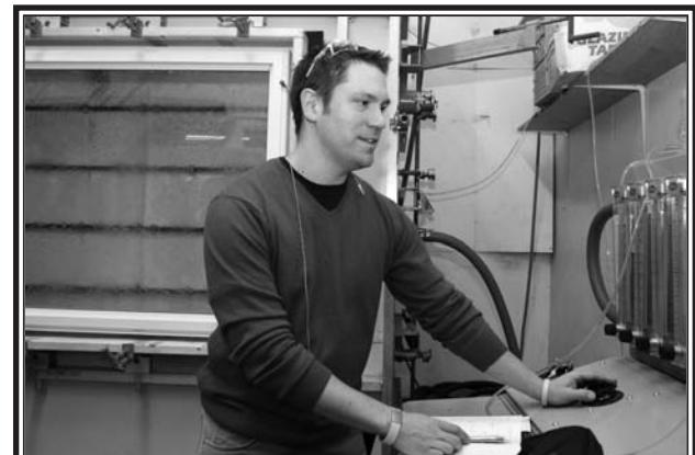
Jeff Addison watches pressure gauges on new structural testing equipment at Kohltech International. The machine tests each newly designed window for water and air leakage to ensure the products are up to Canadian Safety Standards and Environment Canada recommendations. The machine can test wind speeds of up to 500 km/hr. (Harrington Photo)
