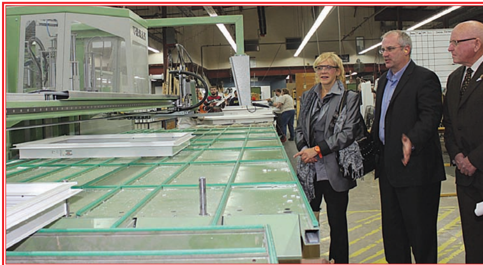
Kohltech International General Manager Kevin Pelley shows MLA Leonore Zann (left) and Major Bob Taylor (right) one of the machines purchased with $65,350 from PIP's Capital Investment Incentive. This machine has automated the cleaning process of manufacturing, rounding out the corners of each window. (Harrington Photo)
