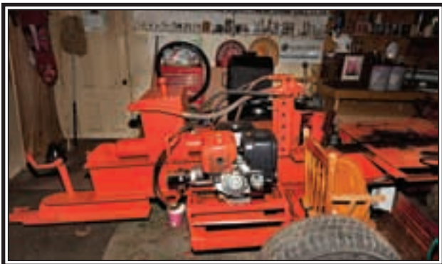
Being the tinkier that he is, Allison MacAleese decided to try his hand at making a log splitter. (Lawrence R. Nicoll Photo)
