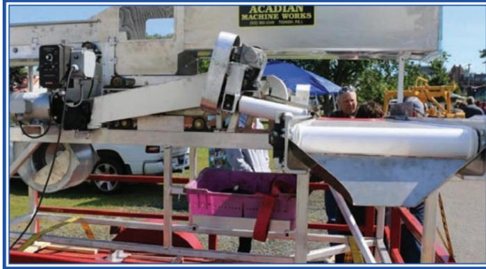
Acadian Machine Works Ltd. has compact cleaning lines that run on 110 volt and can be hauled behind a pick-up truck.
