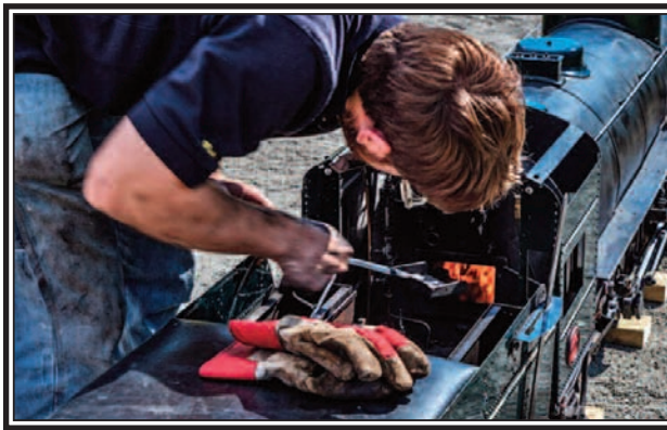
In order for the coal to burn properly in the locomotive, it needs to be stoked, just like a furnace. (Lawrence R. Nicoll Photo)
