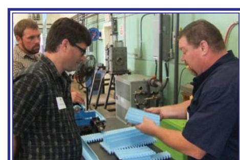
Steve Dormiedy, Plastics Manager, Doug Bragg Enterprises shows off some of the belting designed and manufactured at the Collingwood plant. The facility has two plastic injection machines, one of which is totally automated. Steve says the machine can produce enough belting for the Maritimes blueberry industry in about two months. (Rees Photo)
