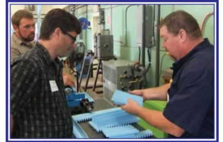
Steve Dormiedy, Plastics Manager, Doug Bragg Enterprises shows off some of the belting designed and manufactured at the Collingwood plant. The facility has two plastic injection machines, one of which is totally automated. Steve says the machine can produce enough belting for the Maritimes blueberry industry in about two months. (Rees Photo)
