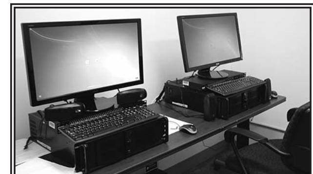
Monitoring station used to record and back-up audio and video interrogations.
