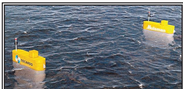
This photo shows the portions of the Tocardo's semi-submersible floating platform which will protrude above the waterline once deployed in Minas Basin (Submitted)
