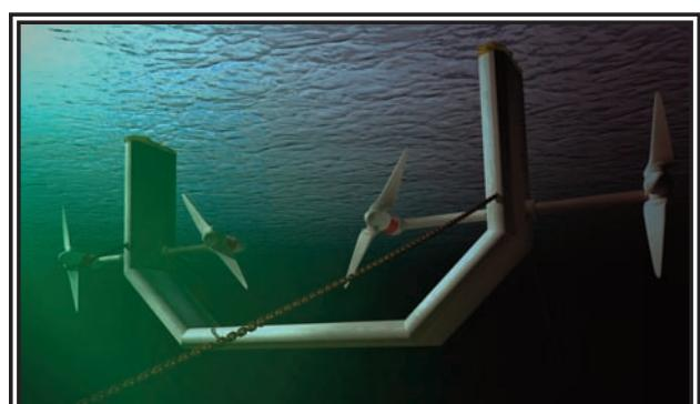
This artist's conception shows what is underwater. Each component will include four 250 Kw T2 bi-directional open rotor turbine generators. Four of these are expected to be installed in the Minas Tidal berth in late 2017. (Submitted)
