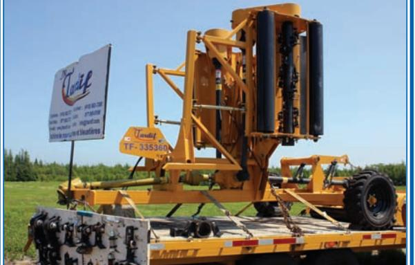
JR Tardif has flail mowers from 4 feet to 16 feet wide. The one on display is a 13 ft model. They also manufacture mulcher and stump-grinding equipment.
