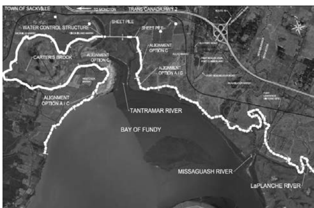
As shown above, Option C (white line) provides a similar construction to Option A with the exception of a new SSP wall, approximately 800 m in length, from the new aboiteaux structure through Tantramar Marsh to Aulac River. A new dyke will be constructed to tie into the existing dyke, which continues to the termination point near Fenton Road.
