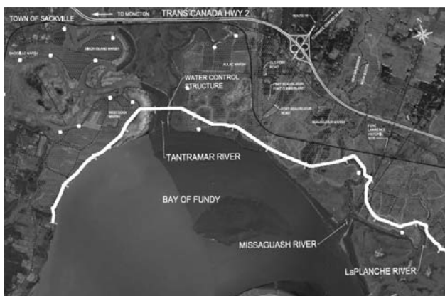
Option B (white line) would include construction of new dykes on the landward side, generally following the existing dyke alignment. The dyke would start south of Sackville and follow existing dyke alignment up to the mouth of the Tantramar River.
