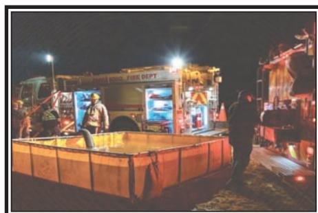
Collapsible water tanks are an important tool for fires in rural areas as shown by its use at cottage fire in Diligent River.
